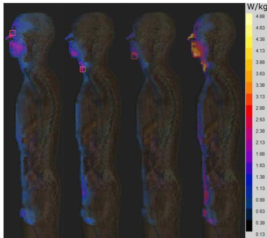
Figure 1: Spatial peak SAR at 30 cm distance from the antennas. From left to right: 900 MHz, 1800MHz, 2100 MHz and combined exposure.
