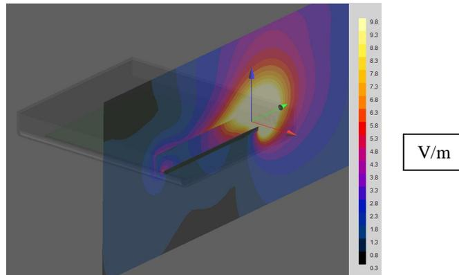
Figure 1: Distribution of Electric field strength (V/m) in the vicinity of the Femtocell.
